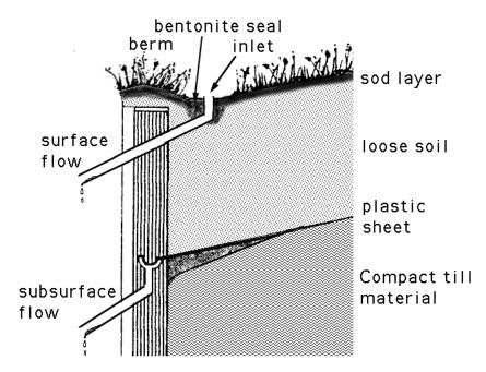
Figure 2-4. Drawing of surface and subsurface flow collectors for use in field sites.
