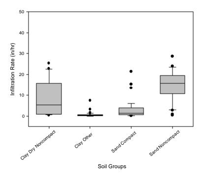
Figure 3-17. Infiltration rates at 120 minutes.
