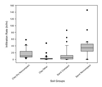
Figure 3-11. Horton's Equation values for initial infiltration - fo.
