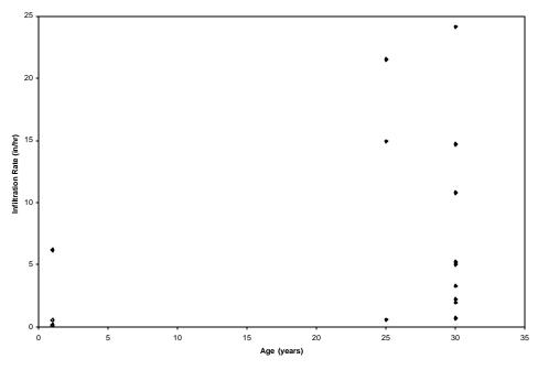
Figure 3-26.  $f_{c}\;\;vs.$  age for dry noncompact clay
