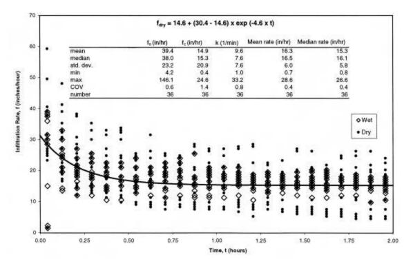
Figure 3-3. Infiltration measurements for noncompacted-sandy soils.
