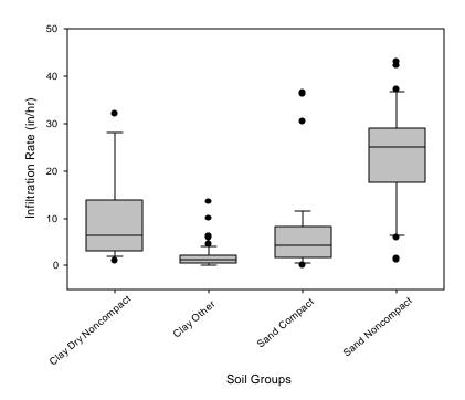
Figure 3-14. Infiltration rates at 15 minutes.
