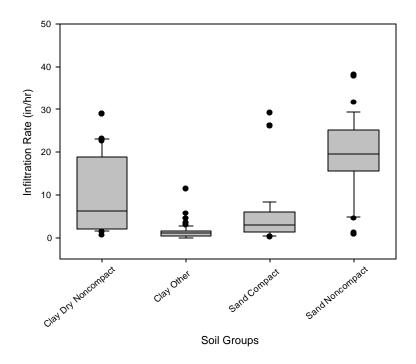
Figure 3-15. Infiltration rates at 30 minutes.
