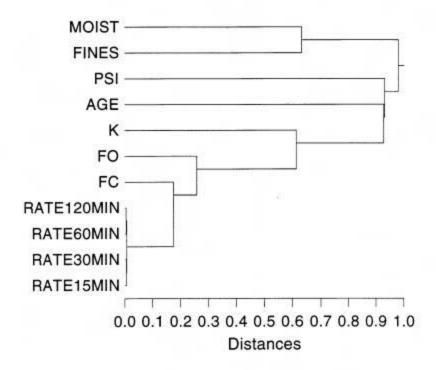
Figure 3-18. Dendogram to investigate complex inter-relationships between site conditions and infiltration parameters.
