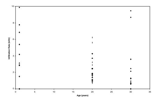
Figure 3-28.  $f_{\rm c}$  vs. age for clay- dry compact, wet compact and wet noncompact.
