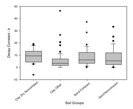
Figure 3-13. Horton's Equation decay constant – k.
