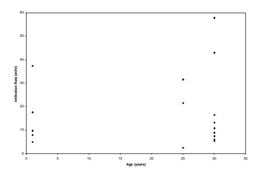
Figure 3-25.  $f_{\text{o}}$  vs. age for dry noncompact clay
