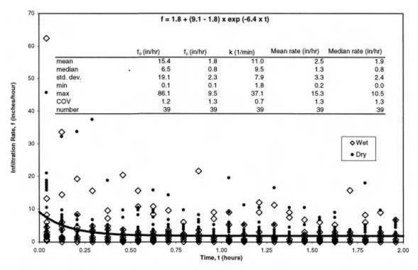
Figure 3-4. Infiltration measurements for compacted-sandy soils.
