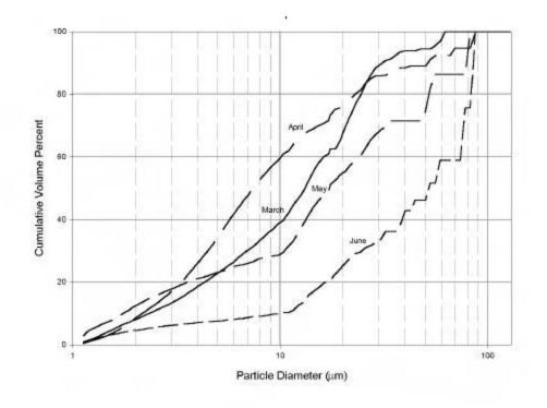
Figure G-1. Particle size for all precipitation samples.
